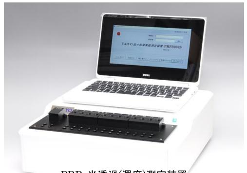
PRP: 光透過(濁度)測定装置 Light Transmission Platelet Aggregometry
